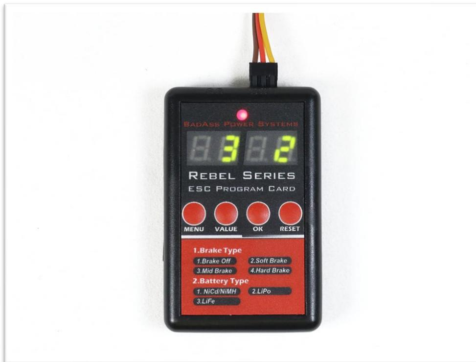
To program this value into the ESC, the OK button is pressed, and that value will be stored in the ESC's memory. This process is repeated for each parameter you wish to change by first pressing the Menu button repeatedly to select the Parameter to be changed, then press the VALUE button repeatedly until the correct option is shown, and finally pressing the OK button once to lock that value into the ESC.
