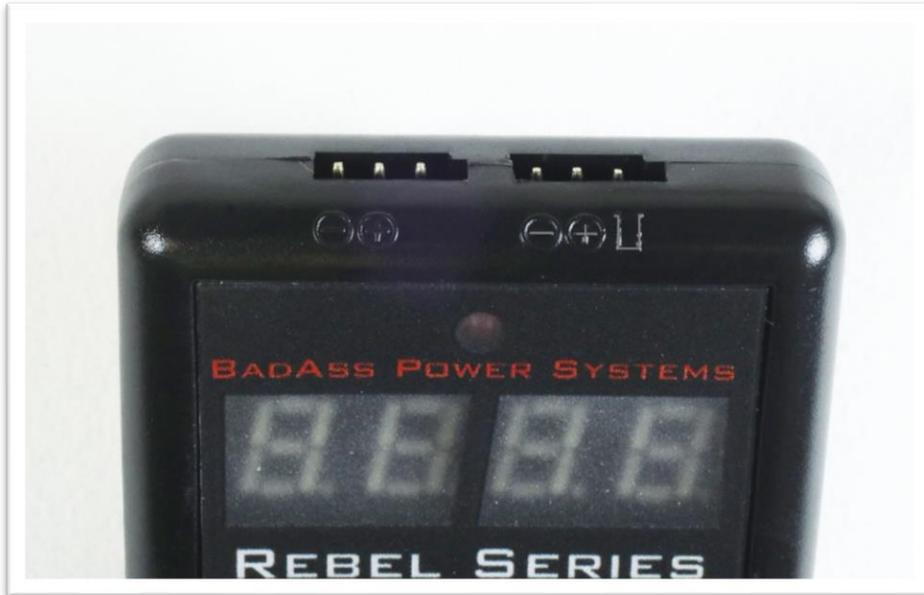
This signifies the wire colors for the control lead when it is plugged in. The “-” indicates the Ground (Brown Wire), the “+” indicates +5 volts (Red Wire) and the “[ ]” indicates the Control Signal (Orange Wire) on the lead. When plugged in it should look like the next photo.
